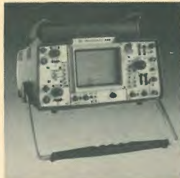
Tektronix 455 Dual Trace Portable Oscilloscope DC-50MHz. 5mV-5V/div. Full delayed sweep. Super condition. £925.00 Large Quantities Available
